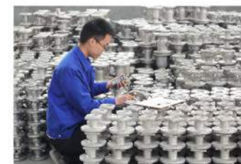
壁厚测试 Wall thickness test
